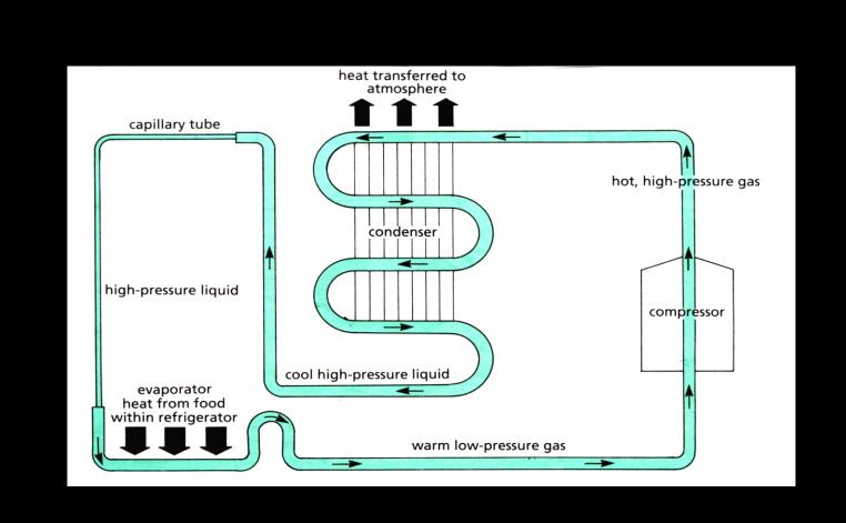
The diagram shows in four stages how the food within a refrigerator keeps in a low temperature.
